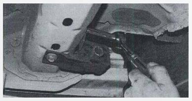
With the cutout made and filed to shape, install the (2) driver side muffler brackets that you purchased. There are threaded holes already in the sub frame for the brackets
