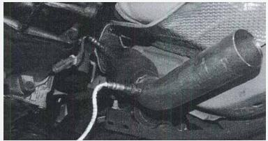
Carefully remove the complete mid pipe section. Install the catted down pipes to the exhaust manifolds, leave slightly loose for adjustment.
