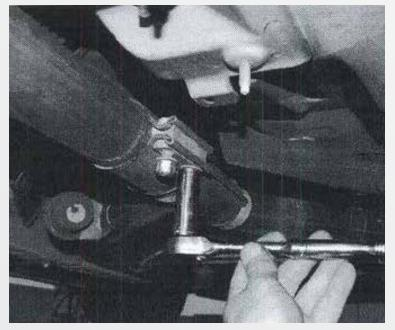
Disconnect all (4) Oxygen Sensors. Loosen and slide back the barrel style clamp at the end of the stock mid pipe section. Remove the hardware at the exhaust manifold collectors for the mid pipe section.
